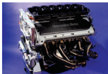
△ 60-degree V12 in the 1997 CLK racer had 592bhp.
